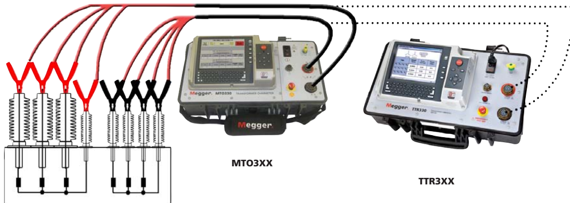
The diagram shows the MTO3xx series and TTR300 series easily and conveniently using the same set of test leads. For example, the user can leave the leads connected to the transformer and use the same lead set to run turns-ratio testing with the Megger TTR3xx series, eliminating several up-and-down-the-ladder trips.
