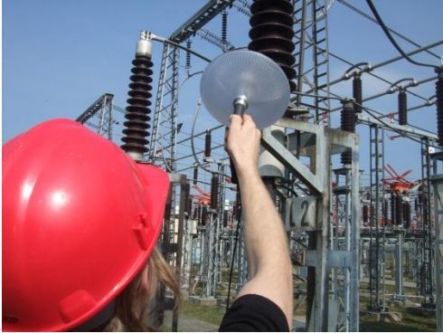
PDS Air™ with Parabolic Acoustic Receiver measuring PD activity in outdoor sealing ends
