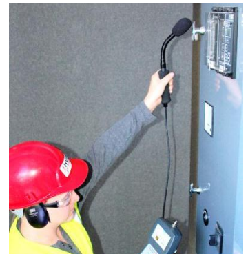
Optional Indoor Acoustic Probe (PDSIAP) in use with Headphones. Outdoor Parabolic Receiver (PDSOPR) also available.
