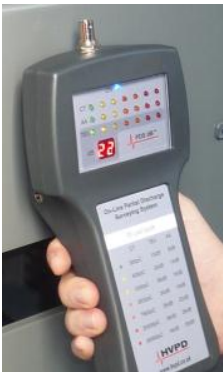
PDS Air™ measuring TEV PD activity in metal-clad air-insulated switchgear
