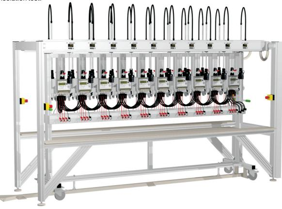
The suspension rack for the isolation can accomodate up to 5 meters. The devices under test are connected via quick connection devices on a conductive aluminium plate by means of a tilting support frame, the status of the device under test can be determined.
