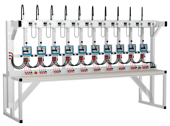
The picture shows a meter test rack with 10 measurement positions. By request different options can be offered to the meter test system:
