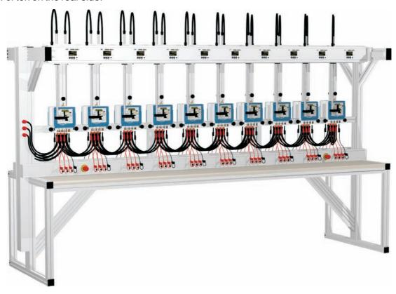
The picture shows a meter test rack for 5 ANSI meters with quick connection devices QCD Form S and isolation current transformers ICT 2.3
