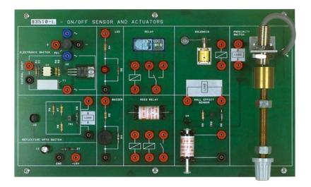
This model includes sensors currently used in industry: an optoelectroreflection barrier, with its output amplifier, a Hall effect sensor with its output amplifier, an inductive proximity sensor with its output amplifier, facing a metallic mass which the operator progressively displaces using a worm screw.
