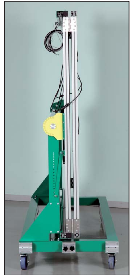
Transport position on wheels. Once the outer panels are folded back and the stabilisers removed, the dimensions are: width 75cm, height 195cm
