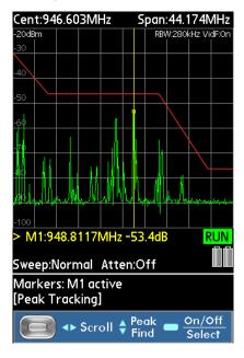
The markers are moved using the navigator keys and can be set to automatically track the peaks.
