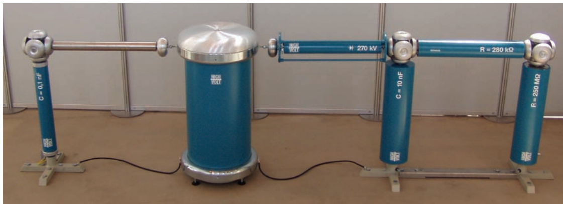
Fig. 5: AC and DC voltage test system 100/135 kV, type WGBS 11/100-135
