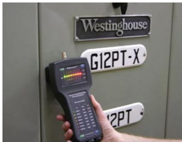
TEV Testing of Solid Insulated Switchgear
