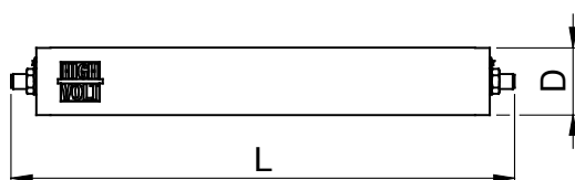
Fig. 6 Schematic sketch of HV resistor
