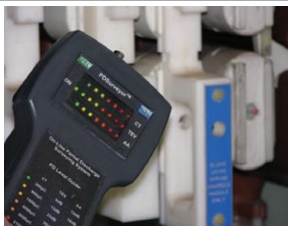
PDSurveyor™ testing AIS for Surface PD
