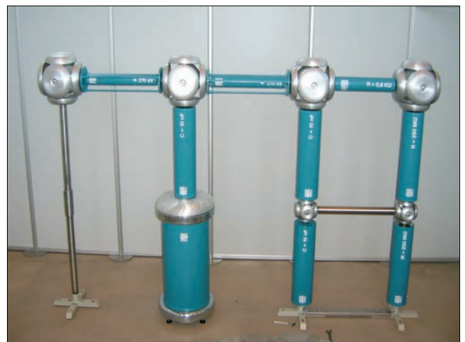
Fig. 3: DC voltage test system 270 kV, type GBS 10/270
