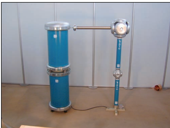
Fig. 1: AC voltage test system 200 kV, type WBS 11/200
