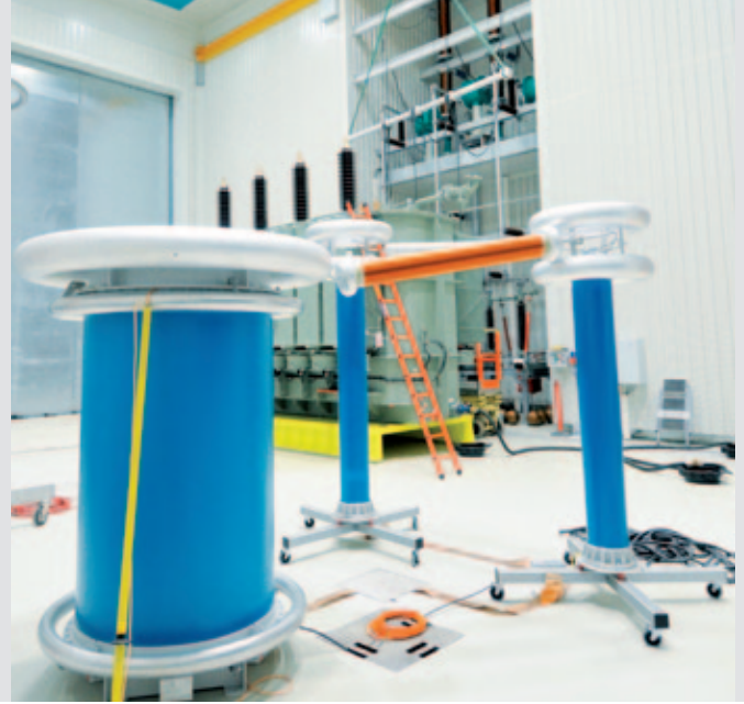
Fig. 2 Applied voltage test system for testing of power transformers, type WRV 5/360 M
