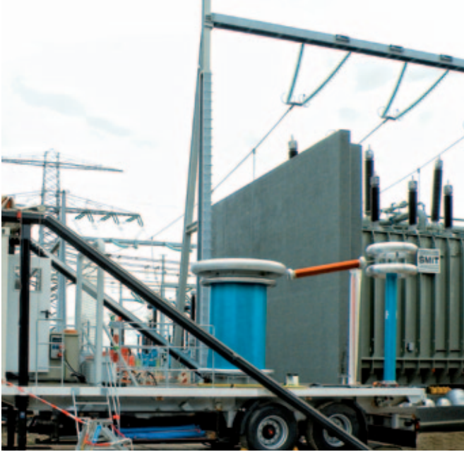
Fig. 1 Applied voltage test system for on-site testing of power transformers, type WRV 5/360 M
